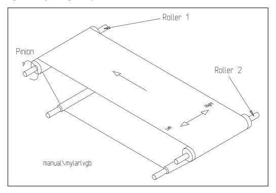
The press is equipped with an automatic belt guard, placed on the guide roller under the follow roller (roller 2).
